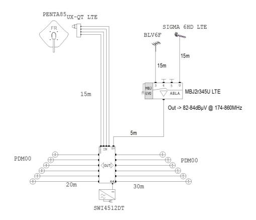
Indication of antennas, antenna holders and preamplifiers from the pole in the scheme is purely indicative, as the choice depends exclusively from the type of TV signal received in the zone of construction of the plant and the structure of the building The present scheme ofproposed maximum does not constitute a project to be drafted by designer enabled.stable. The present scheme of maximum proposed does not constitutes a project that must be drawn up by a qualified designer.
